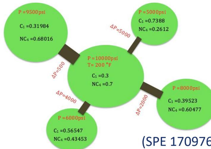
Due to filtration the composition of the fluid may differ in different pores
