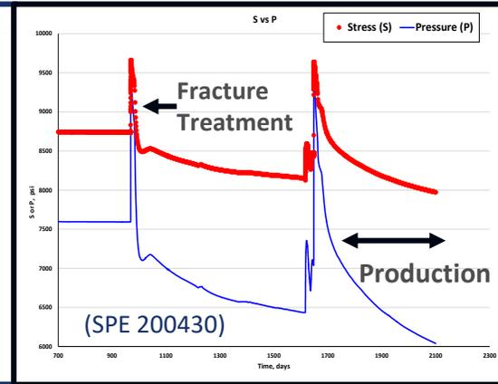
Stress changes during injection as a function of pore pressure
