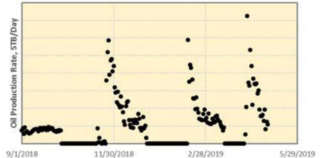
Improved oil production observed by EP Energy after cyclic gas injection in Eagle Ford (SPE 195996)
