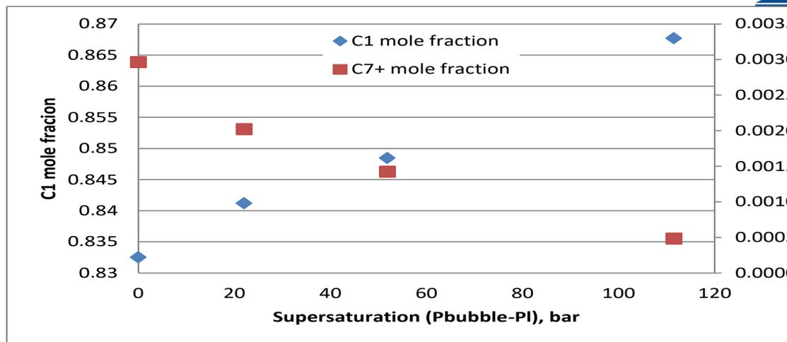
The gaseous phase contains lighter components as the bubble-point suppression increases.
