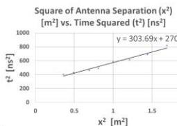
Left, a graph of the square of the antenna separation versus the square of the reflection traveltime from the common midpoint test. The square root of the inverse of the slope gives the half-space velocity which is used for depth conversion
