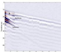
Left, velocity profile created using the common midpoint test. By obtaining a reflection curve from a single horizontal feature, we can model wave velocity through the subsurface.
