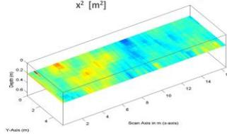
Above, a 3-D model created by interpolating between adjacent GPR profiles. This figure shows a horizontal slice to highlight subsurface features. This manner of viewing GPR data is preferable when seeking objects that span several adjacent profiles.
