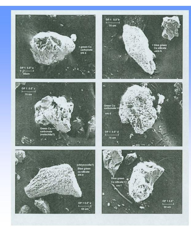
SEM images of copper carbonates and silicates
