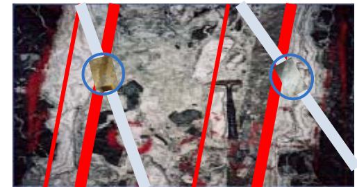
Graphic representation of similar, but smaller, LS veins and stockwork containing abundant coarse Au at McD (McD cores superimposed on Midas, NV, Colorado Grande LS vein ore face)
