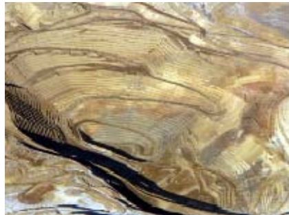
Round Mountain, NV Open Pit: massive, low-grade (0.017opt Au) volcanic-hosted disseminated gold deposit has produced >10Moz in last 20 yrs
