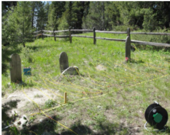
The wood stake is the 13 th electrode, at 6 meters on the results. The line (x=0) starts at the fence on the right (north) and goes south 11.5 meters with an electrode every 0.5 meters. The electrodes are deployed along the tape measure. Note that the next image is looking the other (easterly) direction.
